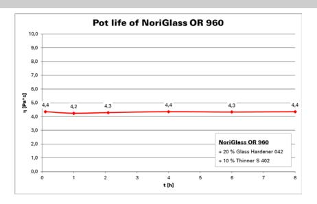
The mixture of ink and glass hardener must be processed within 8 hours.
